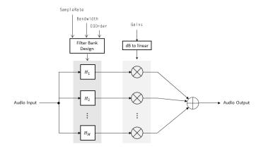
The parallel implementation designs the individual equalizers using the octaveFilter design method and spaces them on the spectrum according to the ANSI S1.11-2004 standard.
