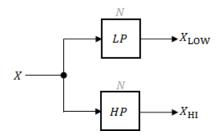
LP and HP are Butterworth filters of order N, implemented as direct-form II transposed second-order sections. The shared cutoff frequency used in their design corresponds to the crossover of the resulting bands.
