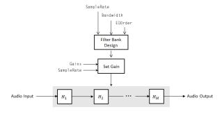
The cascade implementation designs the graphic equalizer filter bank using the multibandParametricEQ System object.
