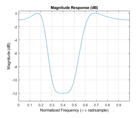
Design a 4th-order lowpass shelving filter with a normalized cutoff frequency of 0.25, a quality factor of 10, and an 8 dB boost gain.
