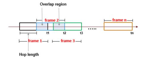
The function computes the mel frequency cepstral coefficients, log energy values, cepstral delta, and the cepstral delta-delta values for each segment as per the algorithm described in cepstralFeatureExtractor System object.
